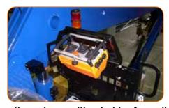
Seat on the column with a holder for radio remote control. Heatable shell seat upon request.
