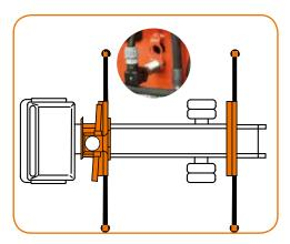
Electr. monitoring of the stabilizing support wide and the slewing range
